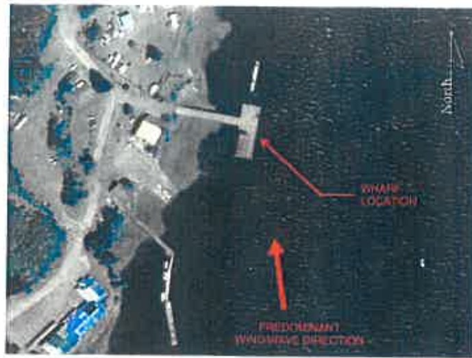
Figure 1 - Wind/Wave Direction on Wharf Structure
